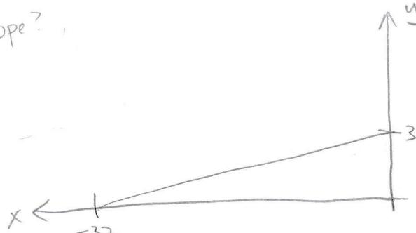
$$\text{Slope } m = \frac{\Delta y}{\Delta x} = \frac{0-3}{-32-0} = -\frac{3}{32} = 0.09375 > 0.0833 = \frac{1}{12}$$
